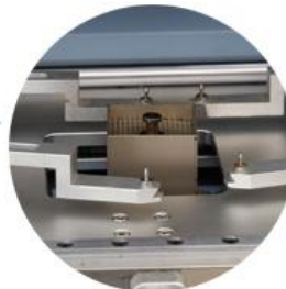
Bottom Heater ( Hot Air 12000w )
